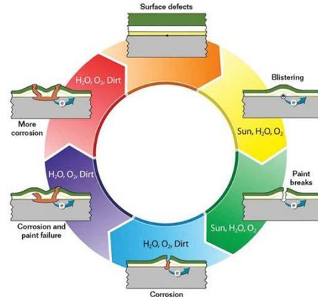
Figure 2. Paint failure and corrosion cycle.
